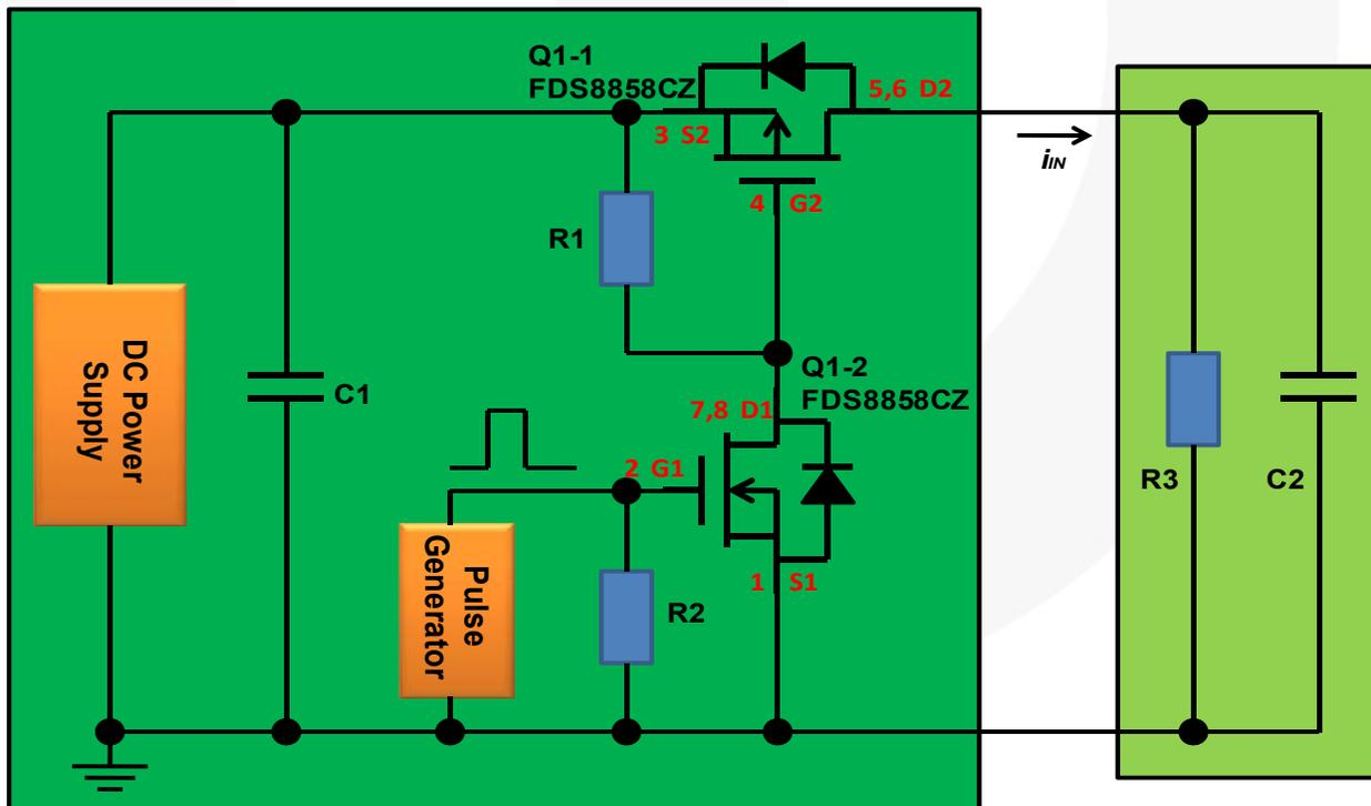
Figure 16. Startup Test Circuit – without FR014H5JZ
