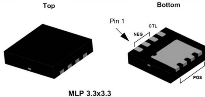
Figure 3. Pin Assignments
