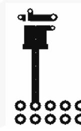
Figure 5. Minimum Pads of 2-ounce Copper
