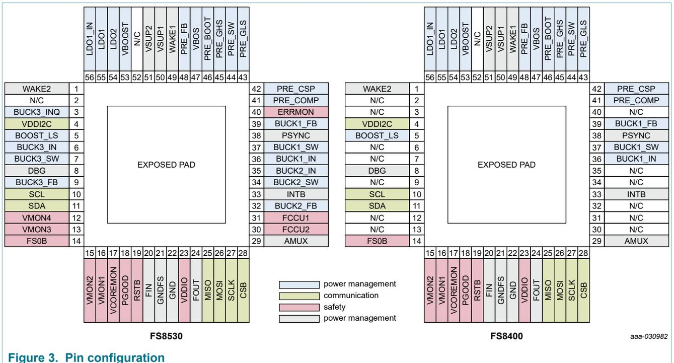
Figure 3. Pin configuration
