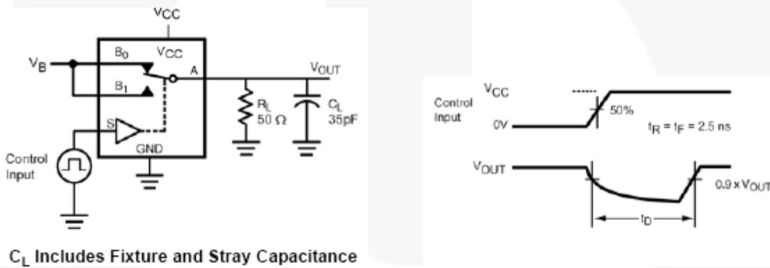
$C_L$  Includes Fixture and Stray Capacitance
