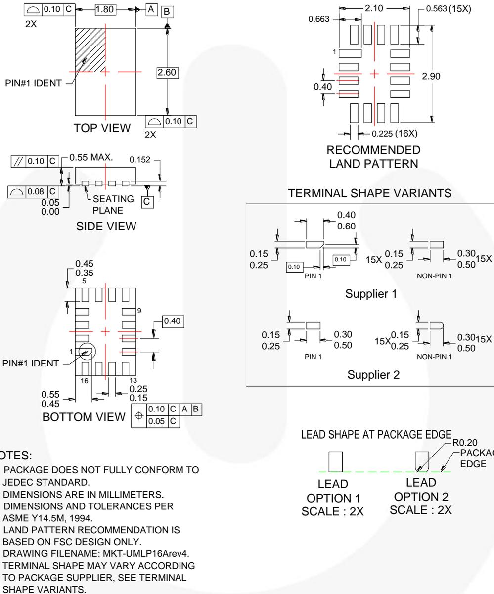
**Figure 16. 16-Lead, Ultrathin Molded Leadless Package (UMLP)**
