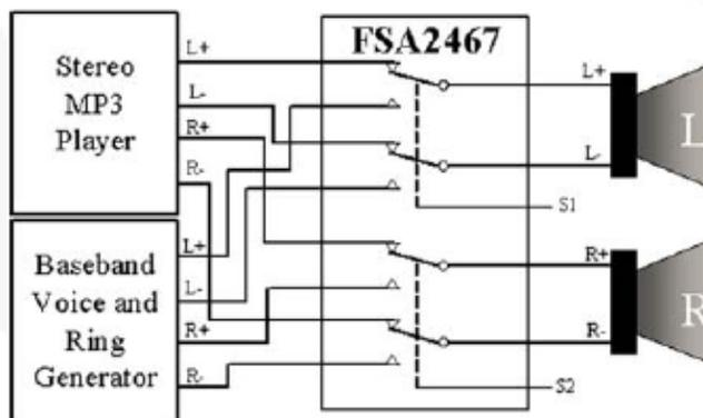
Figure 1. Application Diagram
