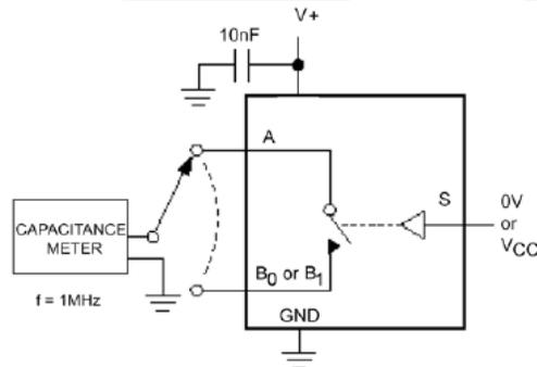
**Figure 12. On / Off Capacitance Measurement Setup**
