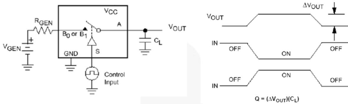
**Figure 11. Charge Injection**
