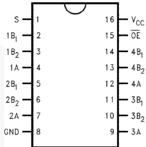
Figure 2. Connection Diagram
