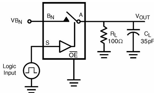
Figure 4.  $t_{on}$ ,  $t_{off}$  Loading
