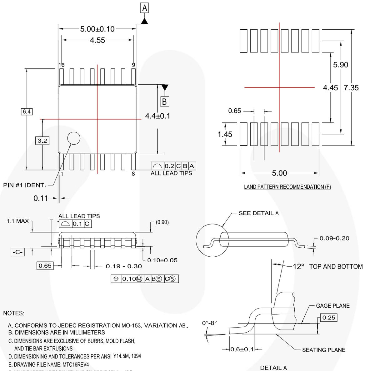
**Figure 7. 16-Lead, Thin Shrink Small Outline Package (TSSOP), JEDEC MO-153, 4.4mm Wide**
