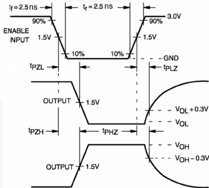
**Figure 4. AC Waveforms**
