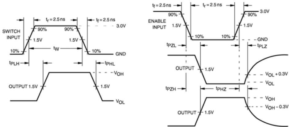
**Figure 4. AC Waveforms**
