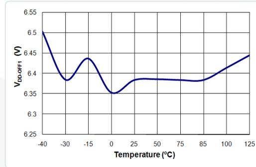
Figure 5. V<sub>DD-OFF1</sub> vs. Temperature
