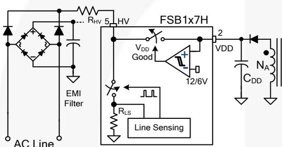
Figure 18. Startup Circuit
