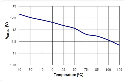
Figure 4. V<sub>DD-ON</sub> vs. Temperature
