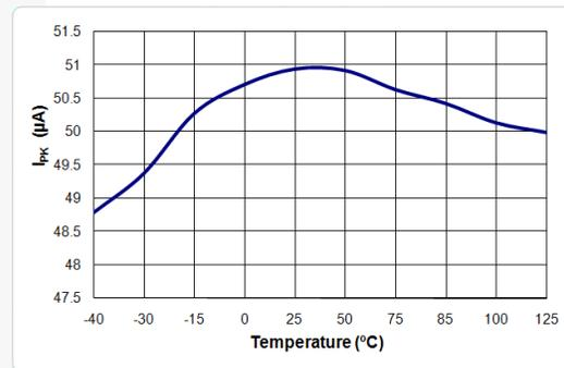
Figure 15. I<sub>PK</sub> vs. Temperature
