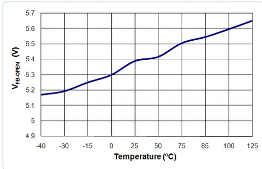
Figure 12. V<sub>FB-OPEN</sub> vs. Temperature
