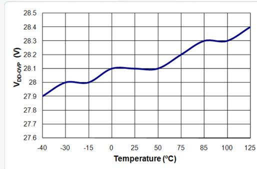
Figure 7. V<sub>DD-OVP</sub> vs. Temperature
