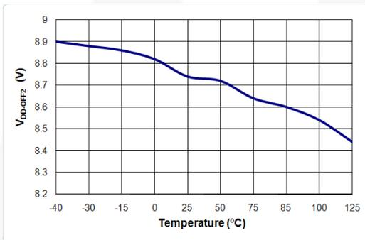
Figure 6. V<sub>DD-OFF2</sub> vs. Temperature
