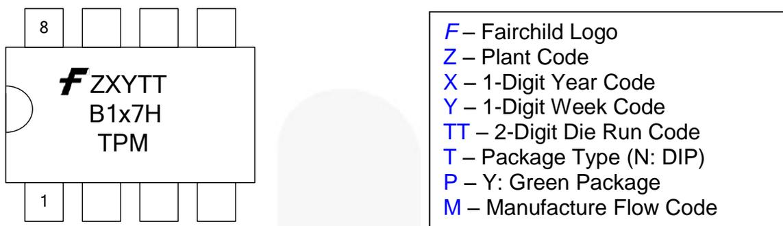
Figure 3. Pin Configuration
