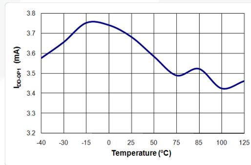
Figure 9. I<sub>DD-OP1</sub> vs. Temperature
