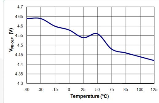
Figure 13. V<sub>FB-OLP</sub> vs. Temperature
