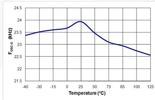
Figure 17. f<sub>osc-G</sub> vs. Temperature
