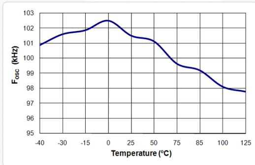
Figure 16. f<sub>osc</sub> vs. Temperature
