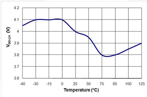
Figure 8. V<sub>DD-LH</sub> vs. Temperature
