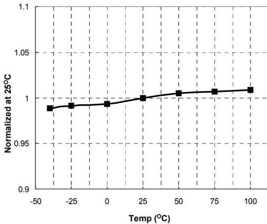
**Figure 14. CON Pin Enable Voltage vs. Temperature**
