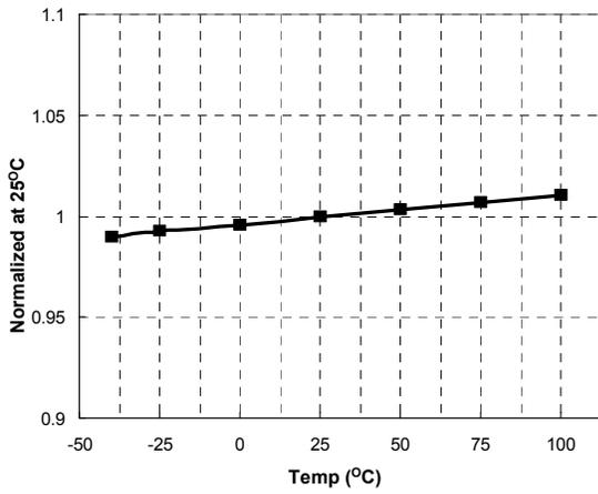
**Figure 12. LV<sub>CC</sub> OVP Voltage vs. Temperature**
