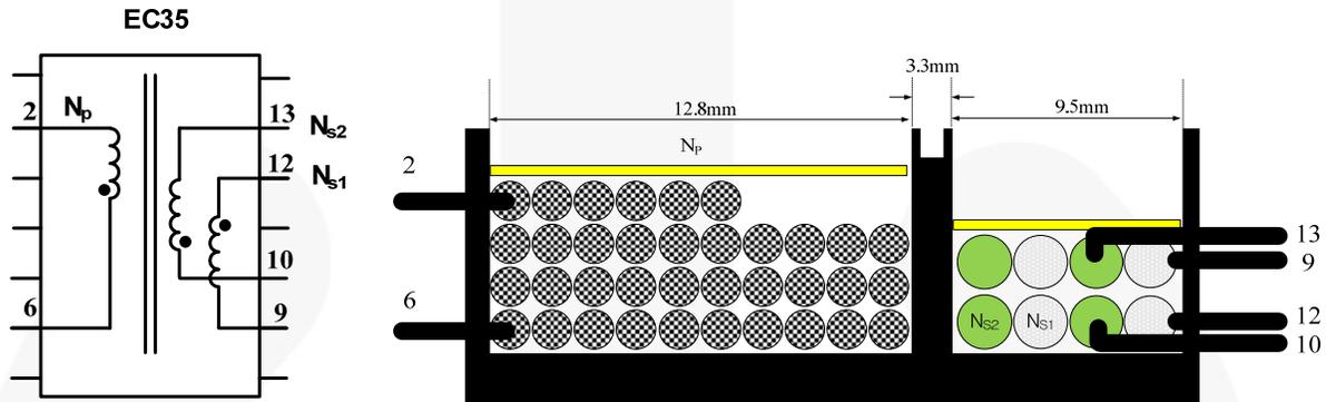
Figure 30. Transformer Construction
