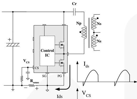
Figure 24. Half-Wave Sensing
