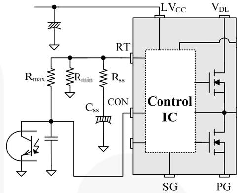
Figure 22. Control Pin Configuration for Pulse Skipping
