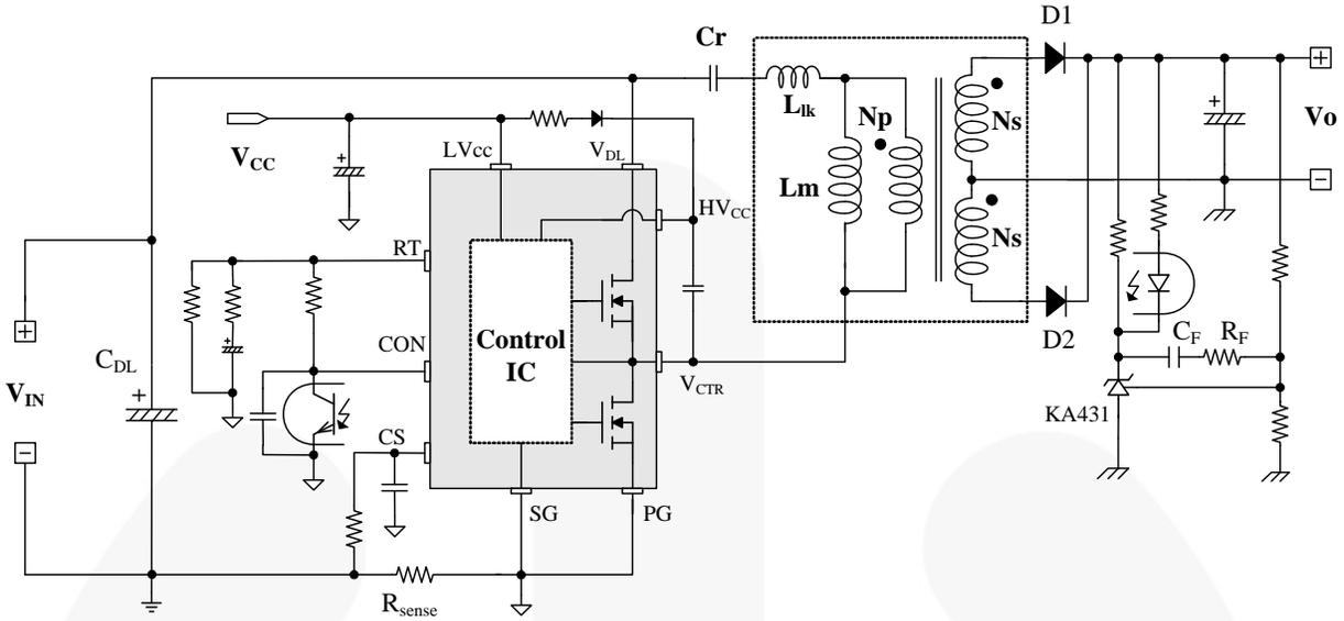
Figure 1. Typical Application Circuit (LLC Resonant Half-Bridge Converter)
