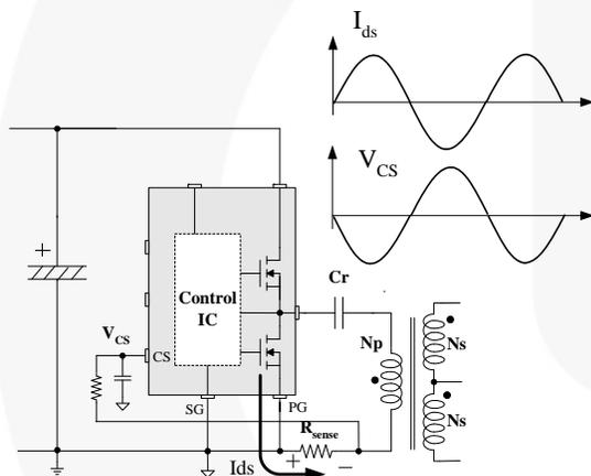
Figure 25. Full-Wave Sensing
