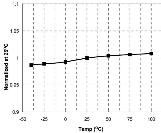
**Figure 13. R<sub>T</sub> Voltage vs. Temperature**
