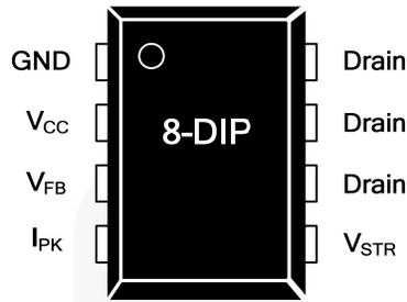
Figure 3. Pin Configuration
