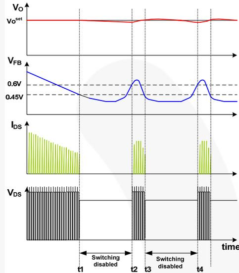
Figure 22. Burst-Mode Operation
