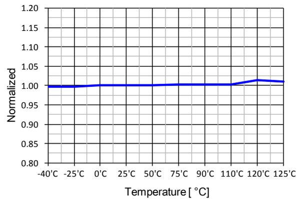
Figure 11. UVLO Threshold Voltage ( $V_{STOP}$ ) vs.  $T_A$
