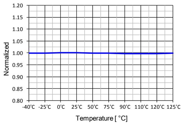
Figure 13. Over-Voltage Protection ( $V_{OVP}$ ) vs.  $T_A$
