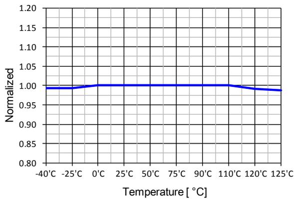
Figure 10. UVLO Threshold Voltage ( $V_{START}$ ) vs.  $T_A$
