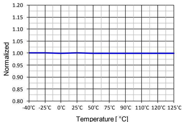
Figure 15. Maximum Duty Ratio ( $D_{MAX}$ ) vs.  $T_A$
