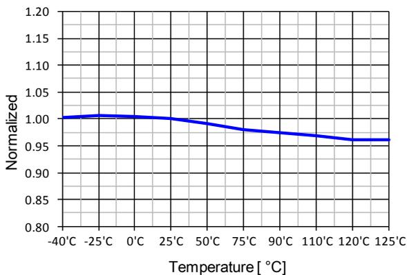
Figure 14. Switching Frequency ( $f_s$ ) vs.  $T_A$
