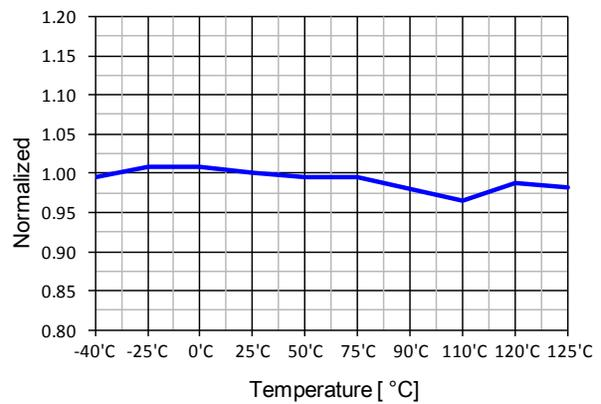
Figure 5. Operating Switching Current ( $I_{OPS}$ ) vs.  $T_A$
