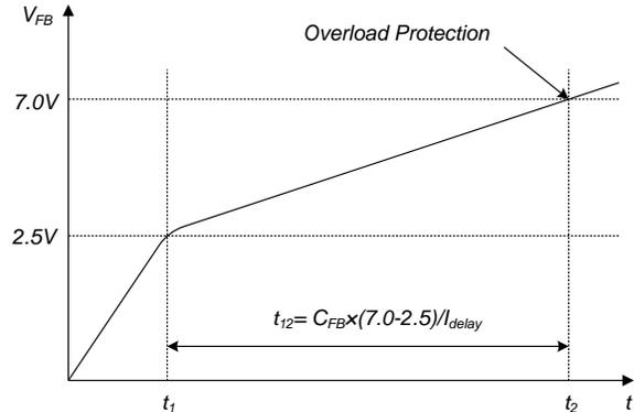
**Figure 21. Overload Protection**
