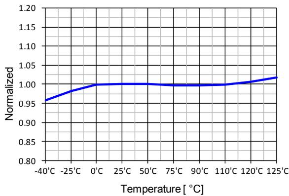
Figure 4. Operating Supply Current ( $I_{OP}$ ) vs.  $T_A$
