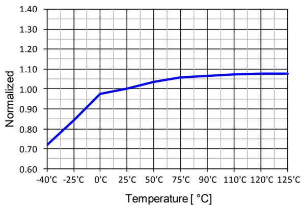
Figure 8. Feedback Source Current ( $I_{FB}$ ) vs.  $T_A$
