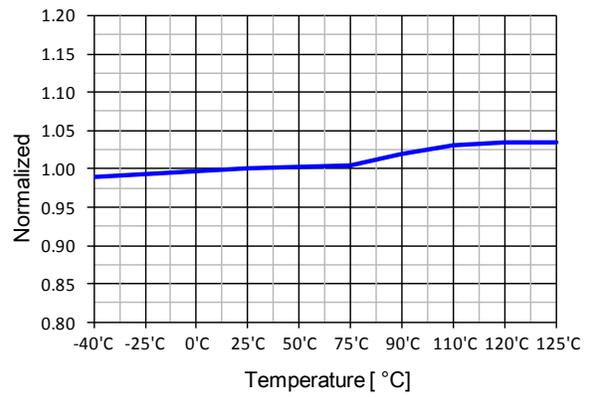
Figure 17. Hysteresis of LOVP ( $V_{INHYS}$ ) vs.  $T_A$
