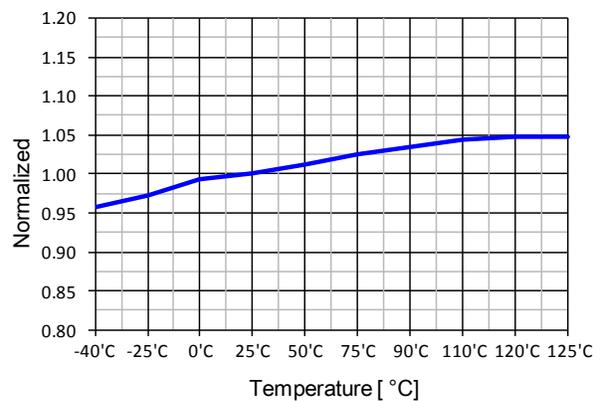
Figure 9. Shutdown Delay Current ( $I_{DELAY}$ ) vs.  $T_A$
