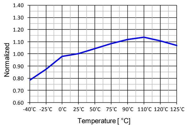
Figure 7. Peak Drain Current Limit ( $I_{LIM}$ ) vs.  $T_A$
