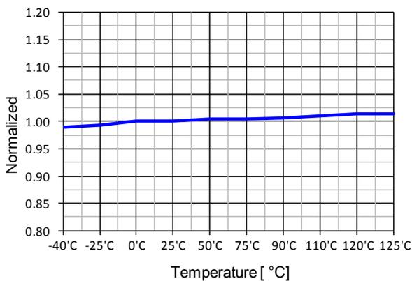
Figure 12. Shutdown Feedback Voltage ( $V_{SD}$ ) vs.  $T_A$
