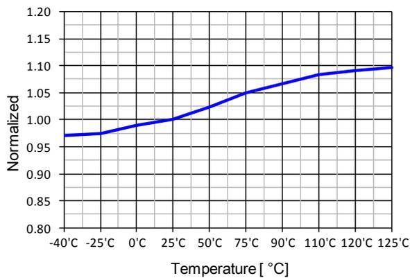
Figure 6. Startup Charging Current ( $I_{CH}$ ) vs.  $T_A$
