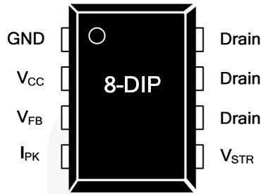
Figure 3. Pin Configuration
