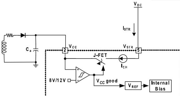
Figure 14. Startup Circuit
