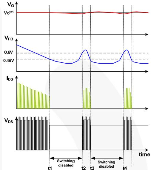
Figure 22. Burst-Mode Operation
