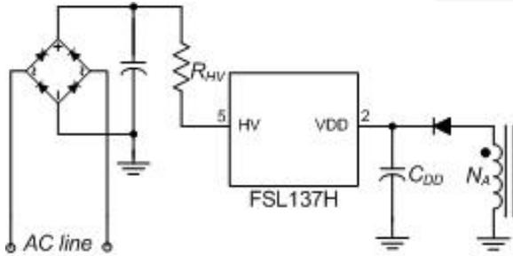
Figure 23. Startup Circuit
