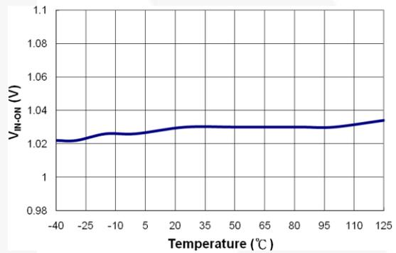
Figure 14. V<sub>IN-ON</sub> vs. Temperature
