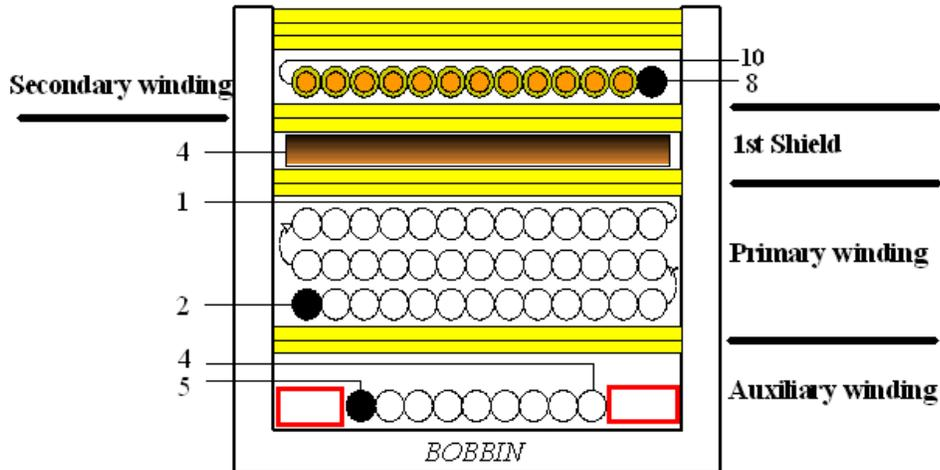
Figure 32. Transformer Diagram
