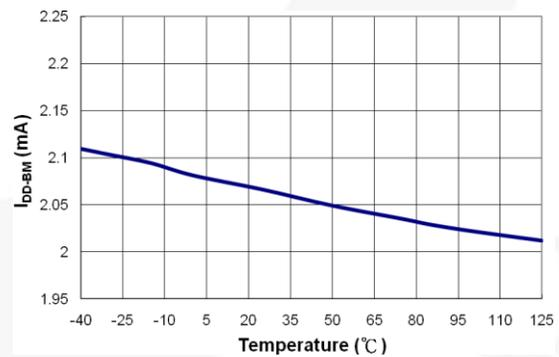
Figure 22. I<sub>DD-BM</sub> vs. Temperature
