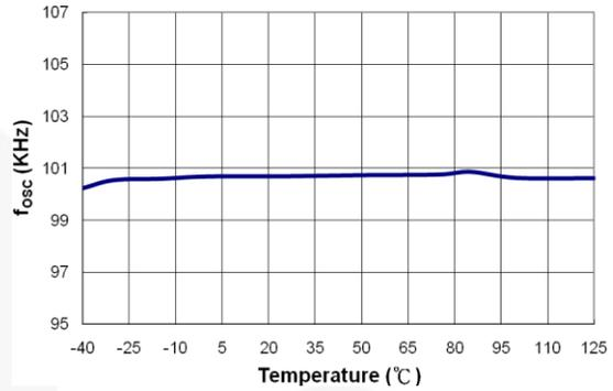
Figure 12. f<sub>osc</sub> vs. Temperature
