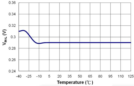
Figure 17. V<sub>IN-L</sub> vs. Temperature
