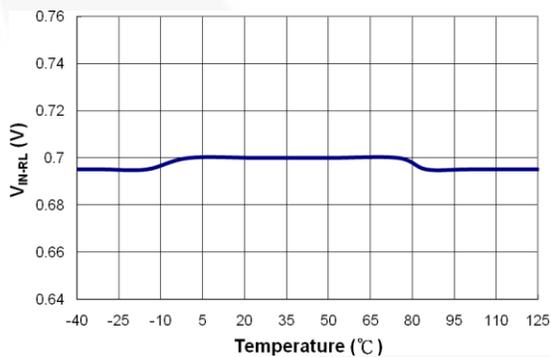
Figure 15. V<sub>IN-RL</sub> vs. Temperature
