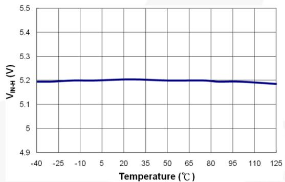
Figure 16. V<sub>IN-H</sub> vs. Temperature
