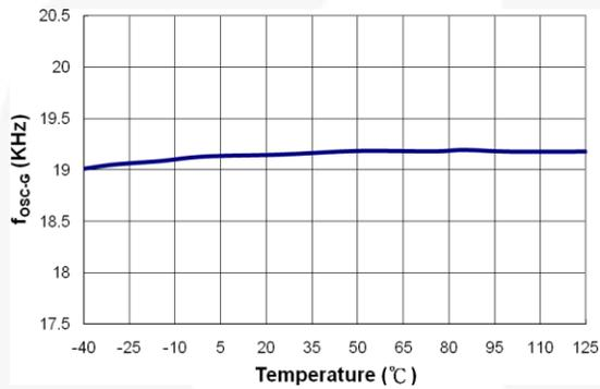
Figure 13. f<sub>osc-G</sub> vs. Temperature
