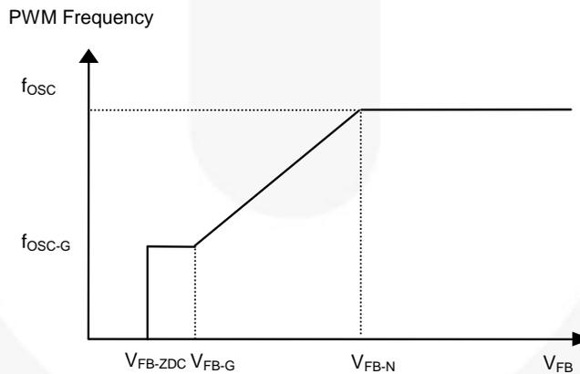
Figure 4. V<sub>FB</sub> vs. PWM Frequency
