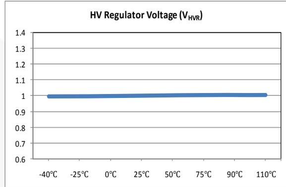
Figure 5. HV Regulator Voltage vs. Temperature
