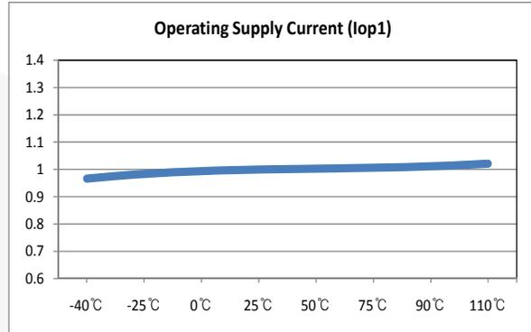
Figure 11. Operating Supply Current 1 vs. Temperature
