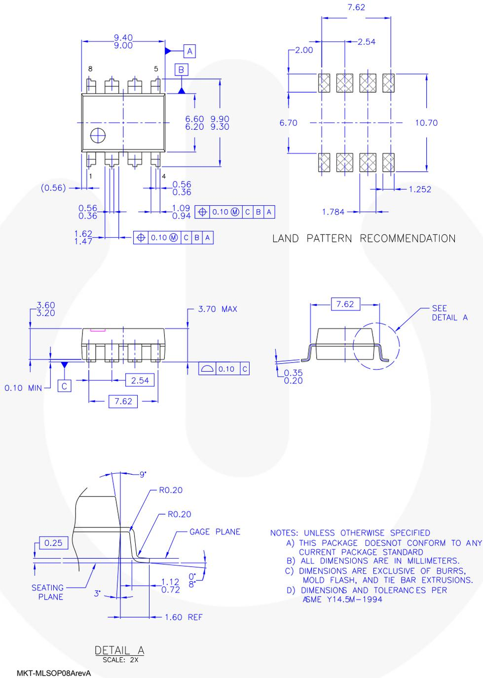
**Figure 25. 8-Lead, .300" Wide, Surface Mount Package (LSOP)**
