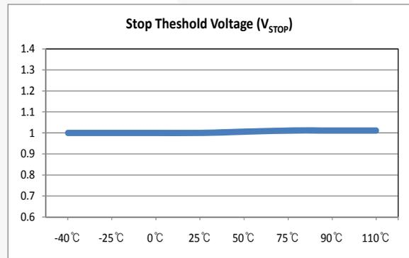
Figure 7. Stop Threshold Voltage vs. Temperature
