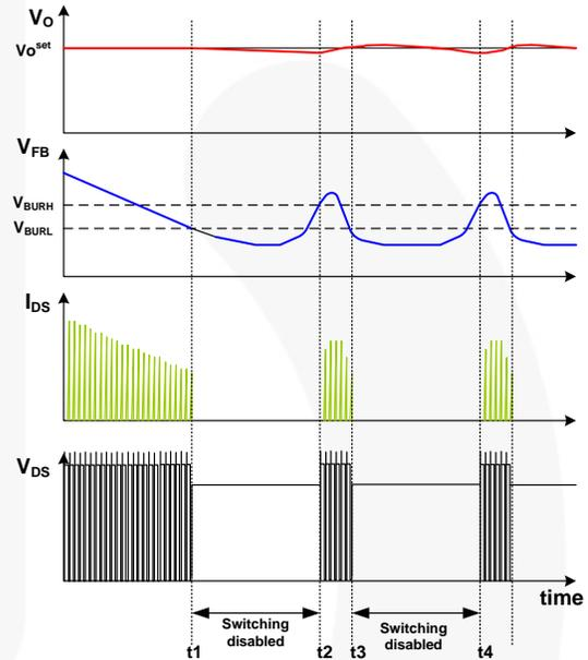
Figure 23. Burst-Mode Operation
