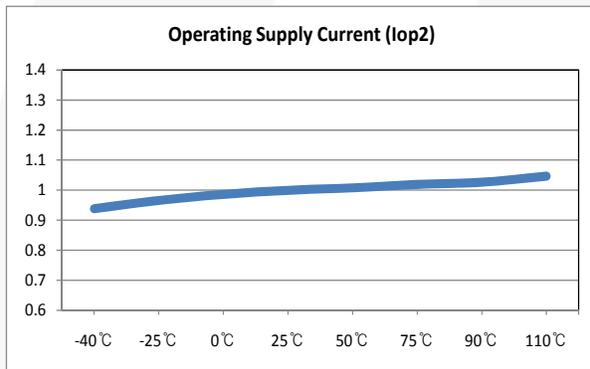
Figure 12. Operating Supply Current 2 vs. Temperature
