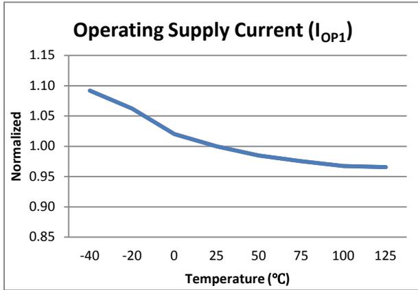
**Figure 11. Operating Supply Current 1 vs. Temperature**
