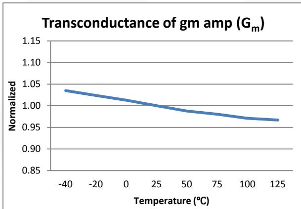
**Figure 13. Transconductance of gm Amplifier vs. Temperature**
