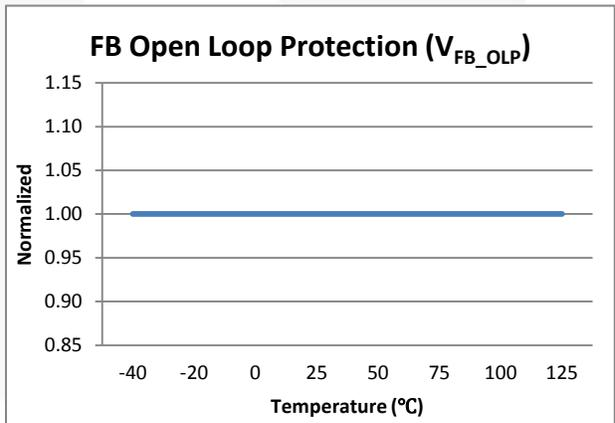
**Figure 14. FB Open Loop Protection Voltage vs. Temperature**
