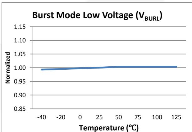
Figure 10. Burst Mode Low Voltage vs. Temperature
