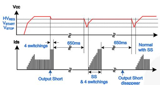
Figure 24. AOCp Waveform
