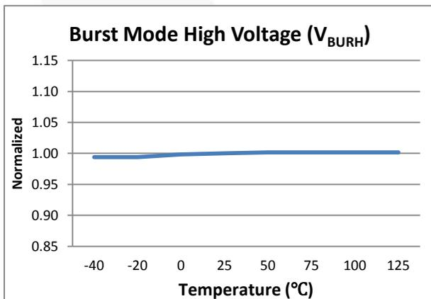
Figure 9. Burst Mode High Voltage vs. Temperature
