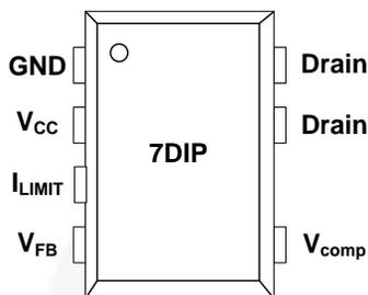
Figure 4. Pin Configuration
