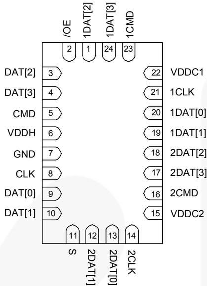
Figure 2. MLP Pin Assignments
