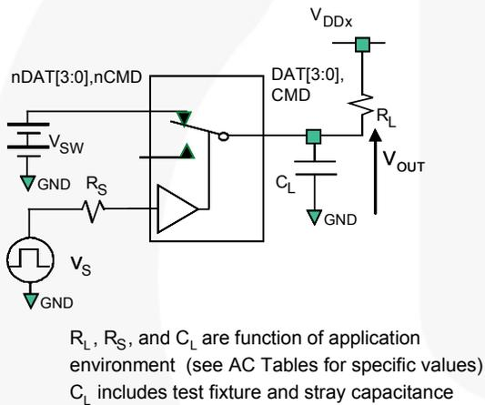
$R_L$ ,  $R_S$ , and  $C_L$  are function of application environment (see AC Tables for specific values)
