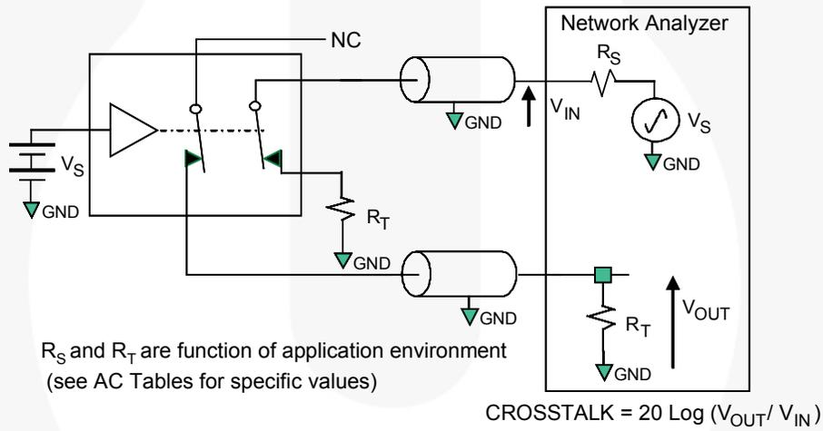
**Figure 13. Channel-to-Channel Crosstalk**
