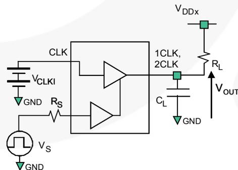
$R_L$ ,  $R_S$ , and  $C_L$  are function of application environment (see AC Tables for specific values)
