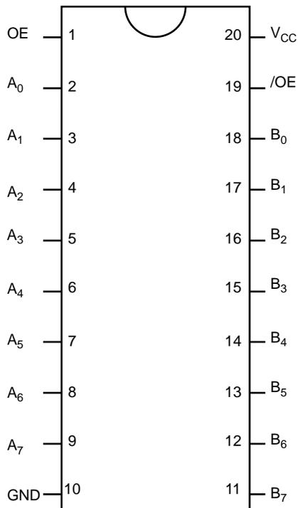
Figure 2. Pin Configuration
