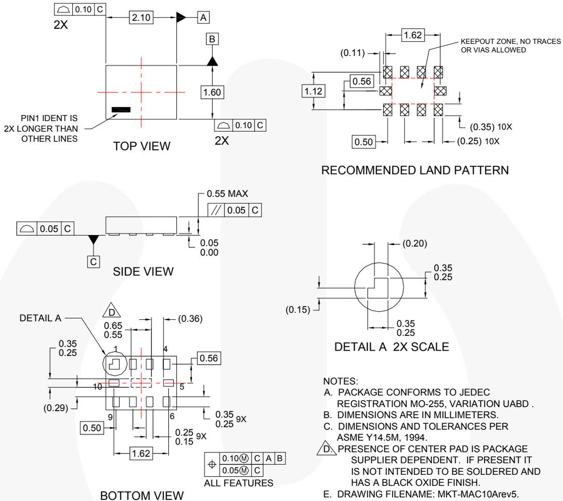
**Figure 13. 10-Lead, MicroPak™, JEDEC MO255, 1.6 X 2.1mm**
