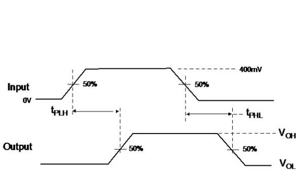
**Figure 10. Propagation Delay ( $t_{rtf} = 500ps$ )**
