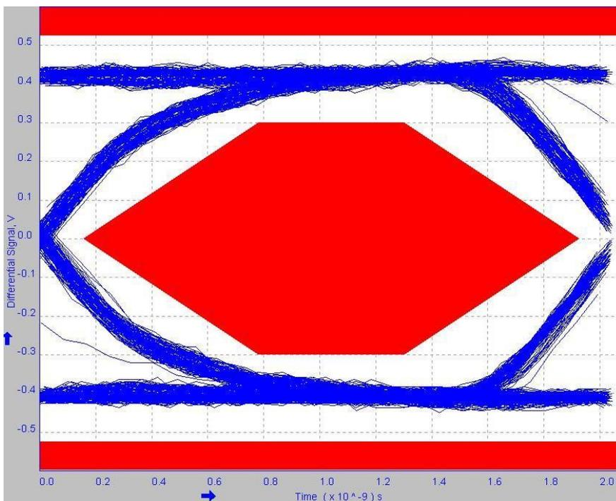
Figure 4. USB 2.0 HS-USB Eye Compliance with Switch
