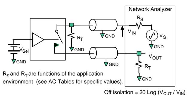
**Figure 14. Channel Off Isolation**
