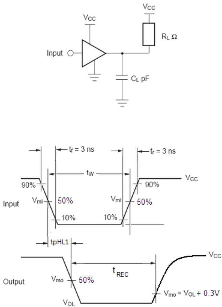
Figure 4. AC Test Circuit and Waveforms for /RST1 Output ST Output
