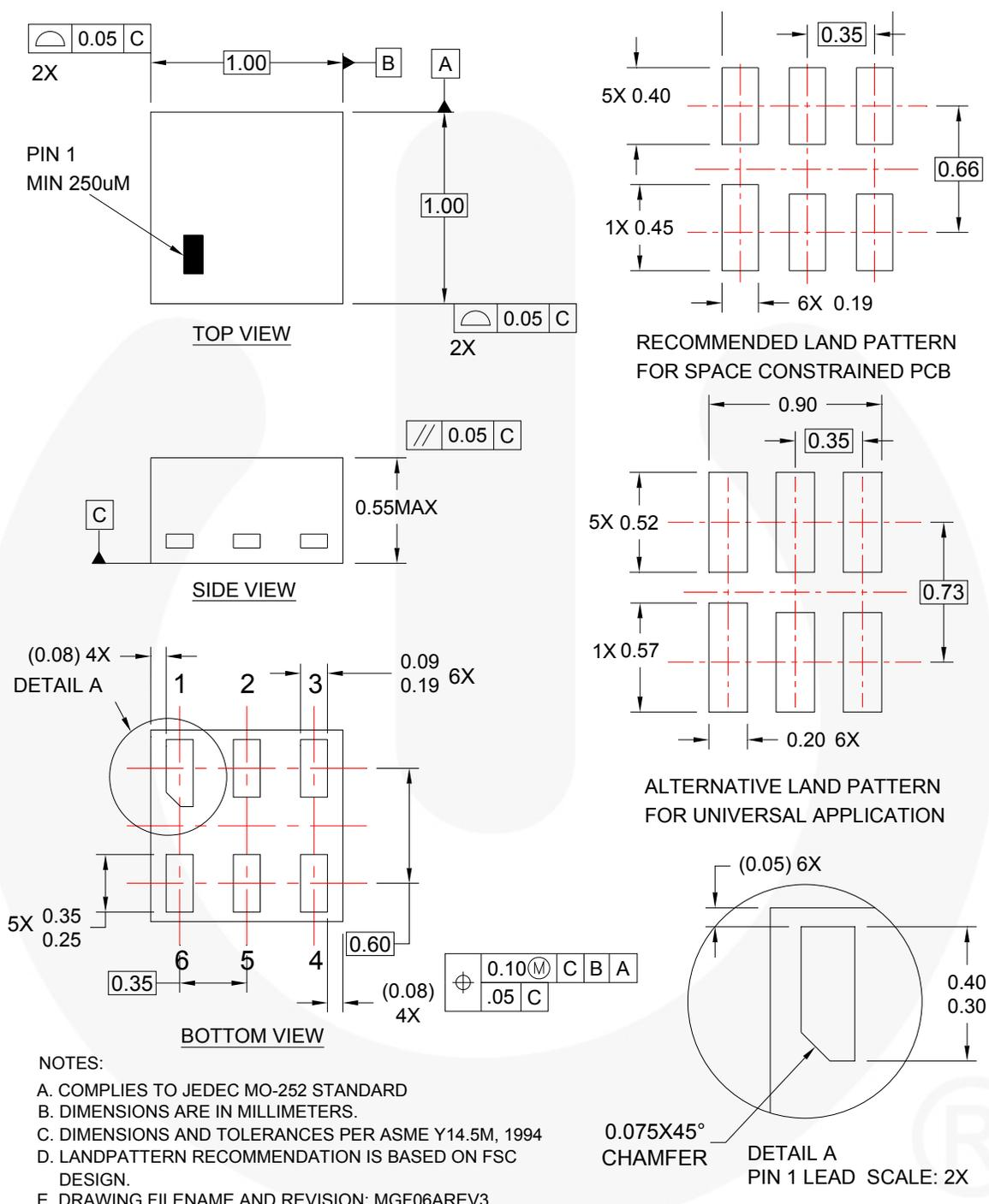
**Figure 6. 6-Lead MicroPak2™ 1.0 x 1.0mm, .35mm Pitch**
