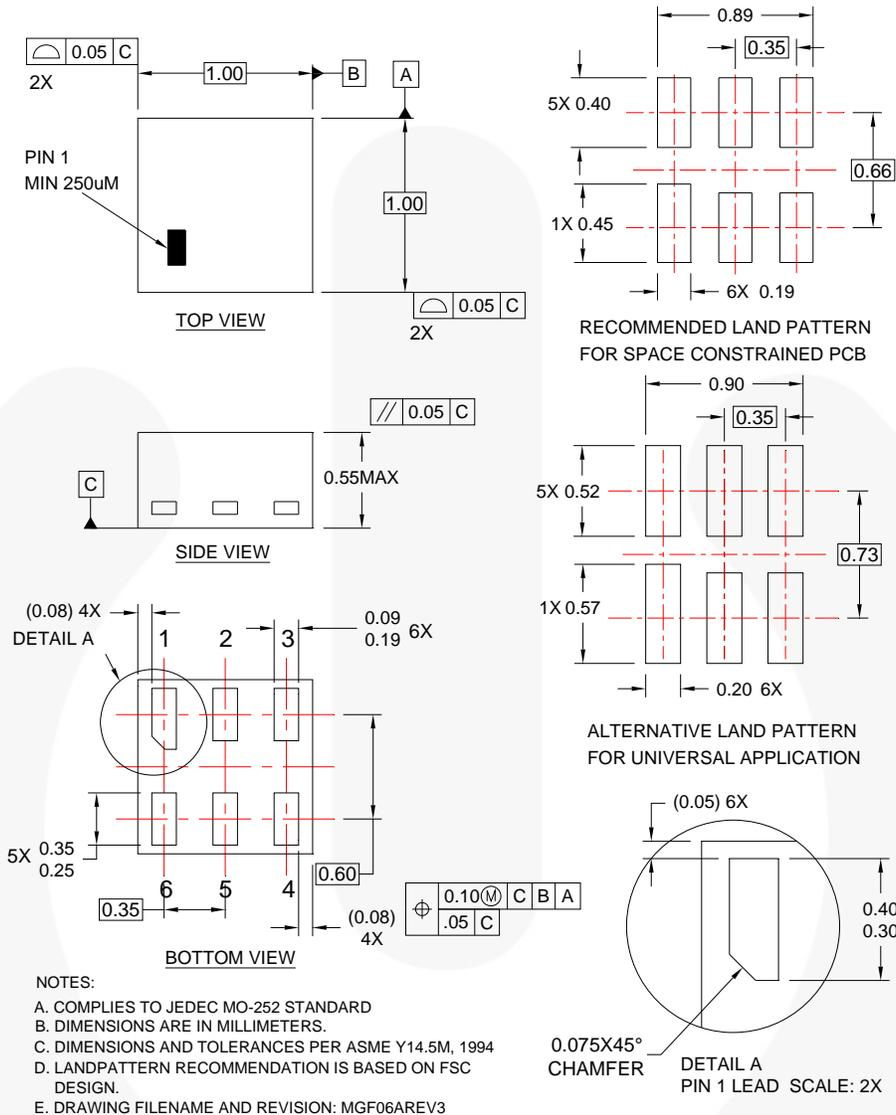
**Figure 7. 6-Lead, MicroPak2™, 1x1mm Body, .35mm Pitch**
