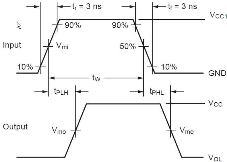
Figure 4. Waveform for Inverting and Non-Inverting Functions
