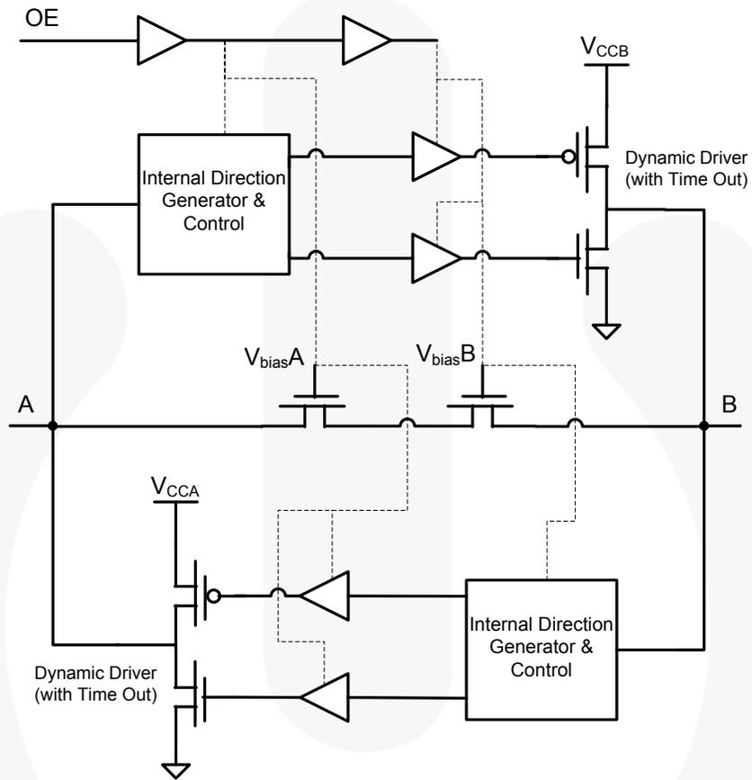
**Figure 1. Block Diagram, 1 of 4 Channels**
