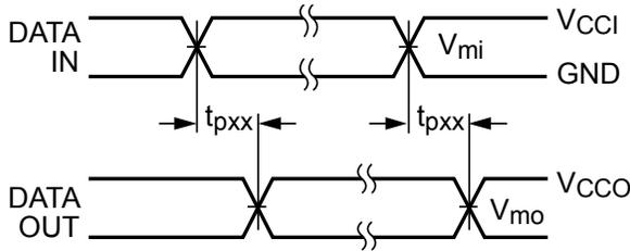
**Figure 8. Waveform for Inverting and Non-Inverting Functions**<sup>(16)</sup>
