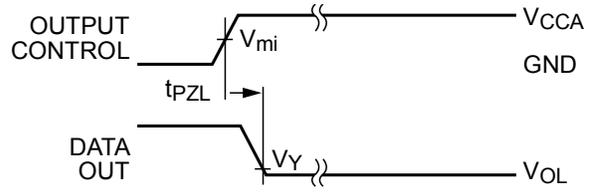
**Figure 9. 3-STATE Output Low Enable Time**<sup>(16)</sup>
