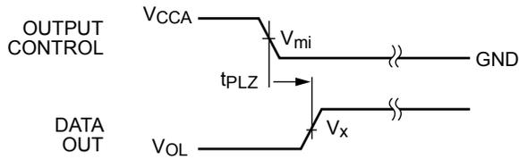
**Figure 10. 3-STATE Output High Enable Time**<sup>(16)</sup>
