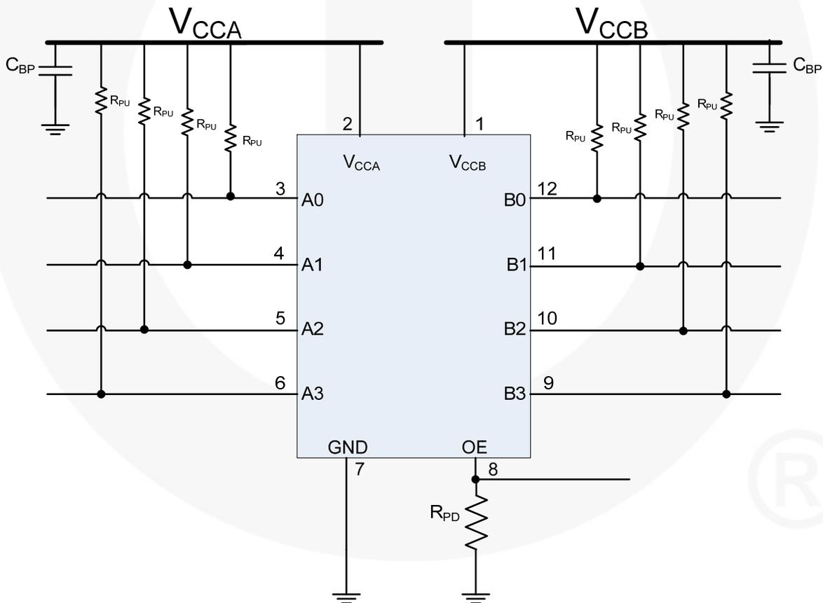
Figure 3. Application Circuit
