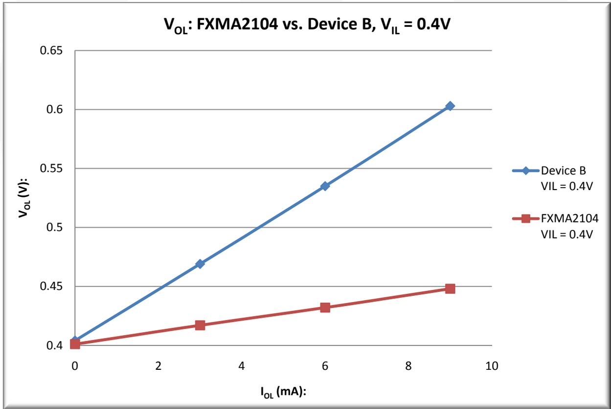
Figure 5. V<sub>OL</sub> vs. I<sub>OL</sub>
