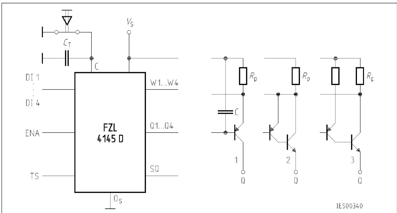
$R_P$  = Precision resistor (current measurement)
