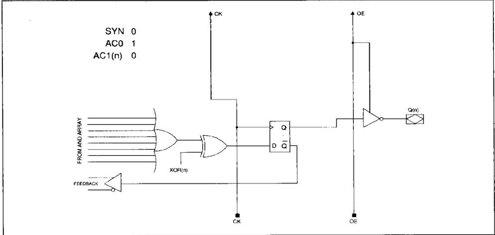
**Combinational Input/Output with Programmable OE and Polarity**
