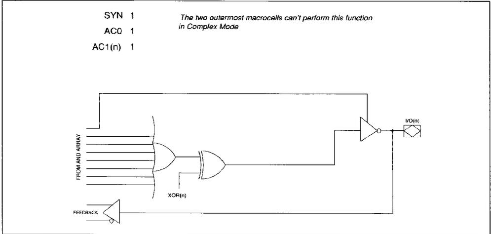
**Combinational Output with Programmable OE and Polarity**
