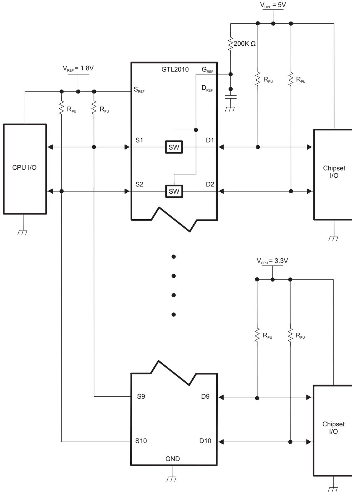
**Figure 5. Bidirectional Translation to Multiple Higher Voltage Levels (Such as an I<sup>2</sup>C or SMBus Applications)**
