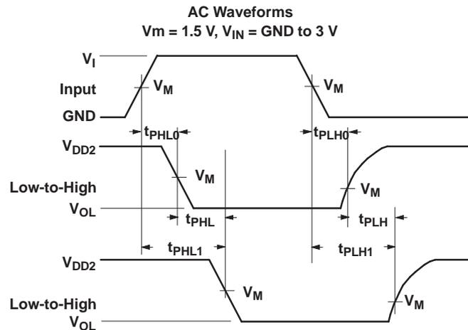
**Figure 1. Input (Sn) to Output (Dn) Propagation Delays**
