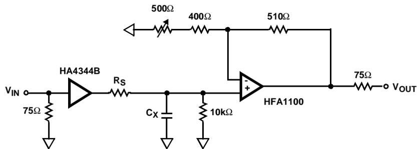
NOTE:  $C_L = C_X + \text{Test Fixture Capacitance}$ .
