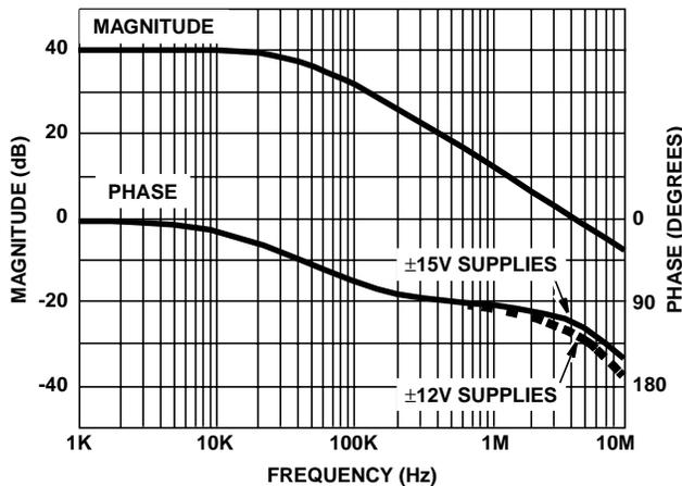
FIGURE 2. MAGNITUDE AND PHASE RESPONSE (CLOSED LOOP GAIN = 100)
