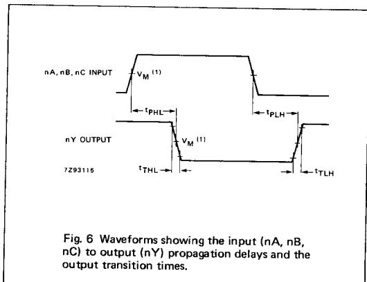
Fig. 6 Waveforms showing the input ( $nA$ ,  $nB$ ,  $nC$ ) to output ( $nY$ ) propagation delays and the output transition times.
