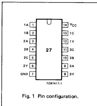
Fig. 1 Pin configuration.
