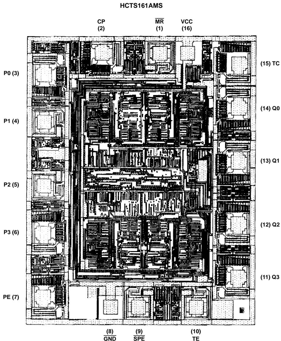
NOTE: The die diagram is a generic plot form a similar HCS device. It is intended to indicate approximate die size and bond pad location. The mask series for the HCTS161A is TA14446A.
