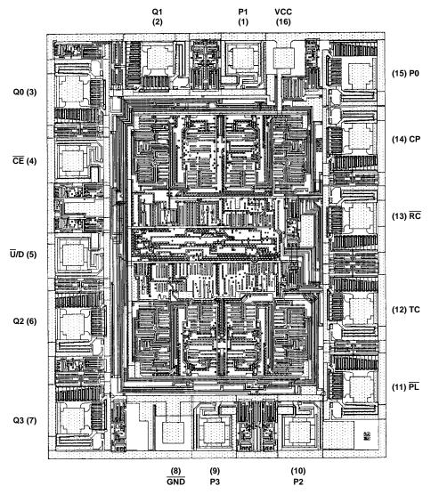
NOTE: The die diagram is a generic plot from a similar HCS device. It is intended to indicate approximate die size and bond pad location. The mask series for the HCTS191 is TA14447A.
