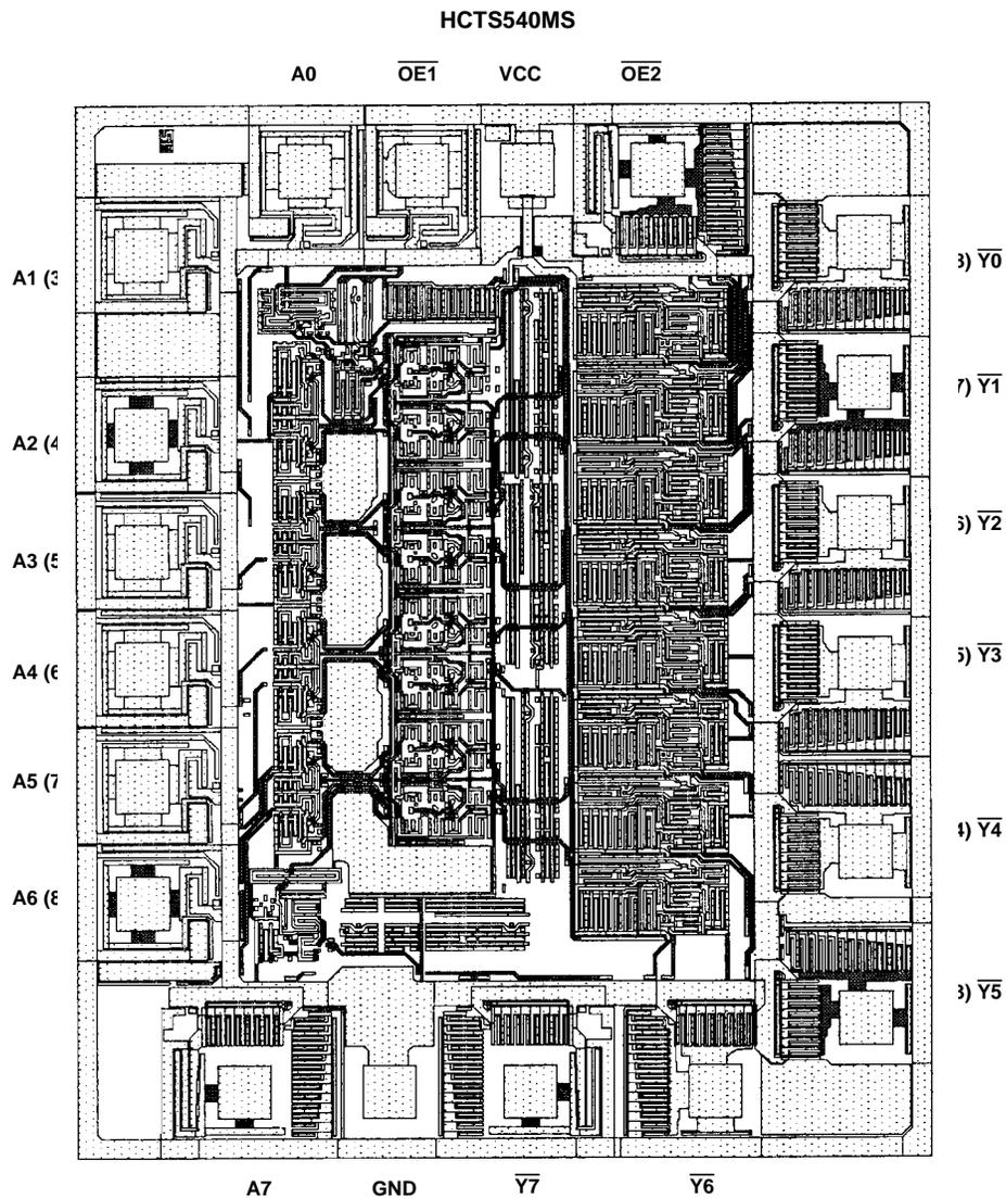
NOTE: The die diagram is a generic plot from a similar HCS device. It is intended to indicate approximate die size and bond pad location. The mask series for the HCTS540 is TA14455A.
