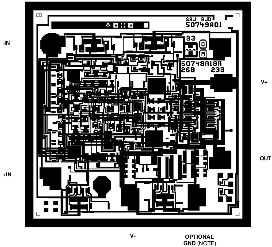
NOTE: This pad is not bonded out on packaged units. Die users may set a GND reference, via this pad, to ensure the TTL compatibility of the DIS input when using asymmetrical supplies (e.g. V+ = 10V, V- = 0V).
