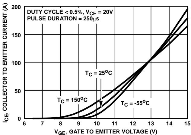
FIGURE 13. TRANSFER CHARACTERISTIC
