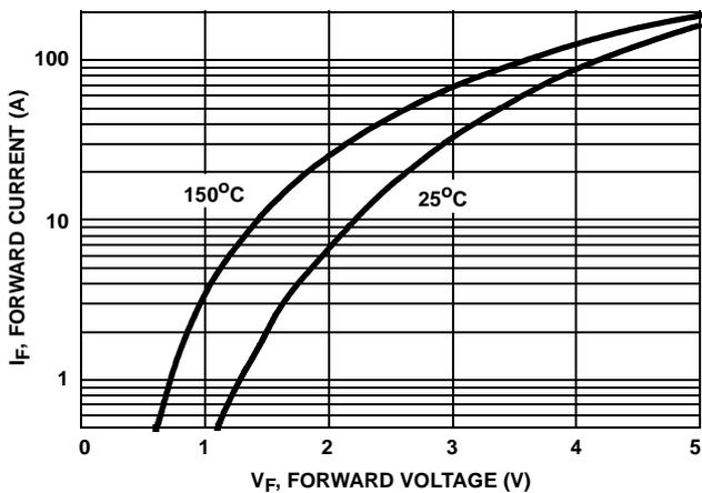
FIGURE 18. DIODE FORWARD CURRENT vs FORWARD VOLTAGE DROP
