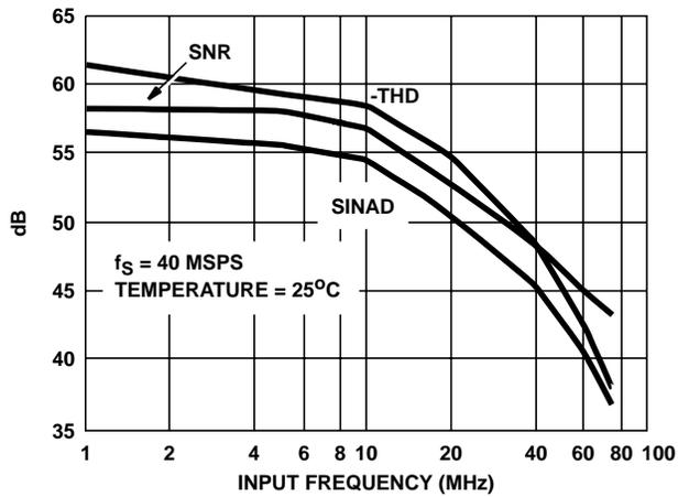
FIGURE 5. SINAD, SNR, AND -THD vs INPUT FREQUENCY
