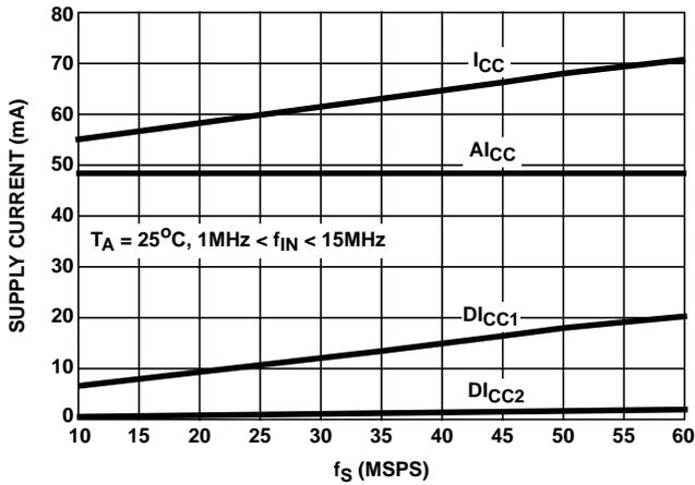
FIGURE 8. SUPPLY CURRENT vs SAMPLE CLOCK FREQUENCY
