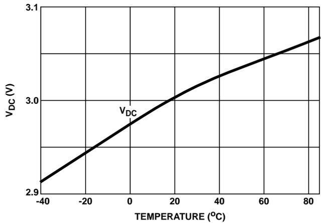
FIGURE 11. DC BIAS VOLTAGE ( $V_{DC}$ ) vs TEMPERATURE
