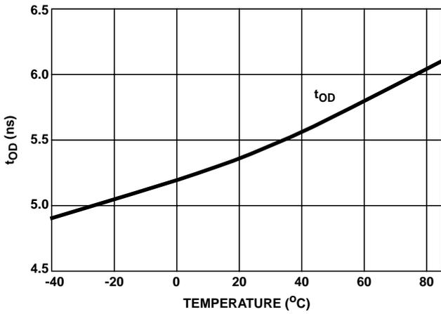
FIGURE 12. DATA OUTPUT DELAY ( $t_{OD}$ ) vs TEMPERATURE
