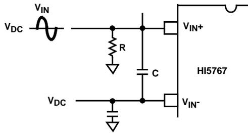
FIGURE 19. DC COUPLED SINGLE ENDED INPUT
