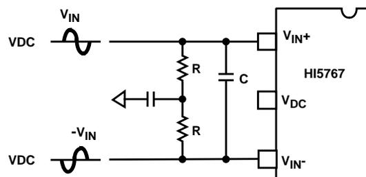
FIGURE 17. DC COUPLED DIFFERENTIAL INPUT
