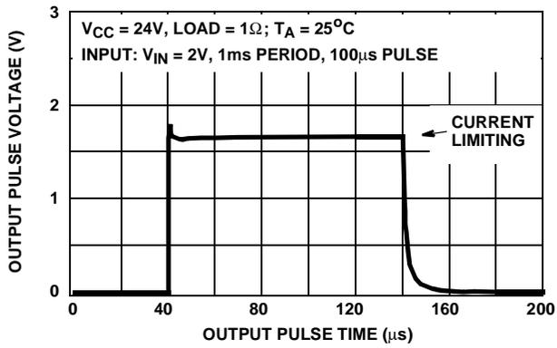
FIGURE 7. TYPICAL OUTPUT CURRENT PULSE WHEN SWITCHING INTO A LOW IMPEDANCE ( $1\Omega$ ), OR SHORTED LOAD. FOR THE CONDITIONS SHOWN, OUTPUT CURRENT LIMITING IS  $\sim 1.7\text{A}$
