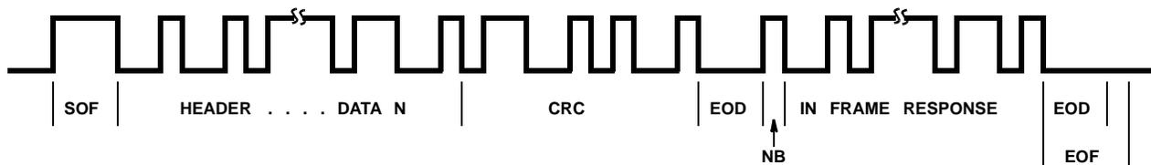
FIGURE 5. J1850 MESSAGE WITH IN-FRAME-RESPONSE
