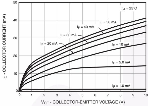
Fig. 7 Collector Current vs. Collector-Emitter Voltage
