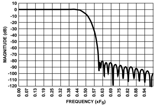
FIGURE 13. DIGITAL-TO-ANALOG FREQUENCY RESPONSE (FULL SCALE INPUTS, 0dB)
