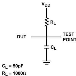
**Three-State High Load Circuit**
