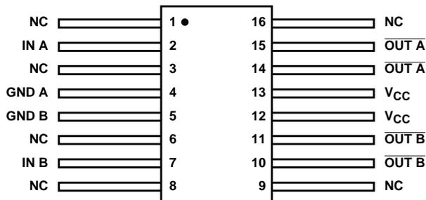
NOTE: Pins 4 and 5, 10 and 11, 12 and 13, 14 and 15 are double-bonded to their same electrical points on the die.
