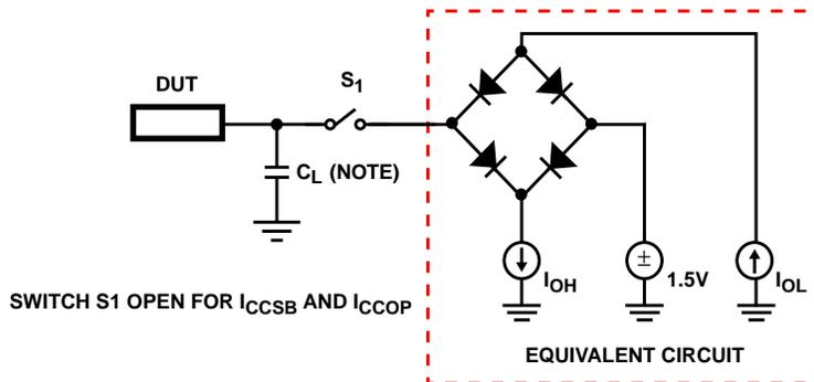
NOTE: Test head capacitance.
