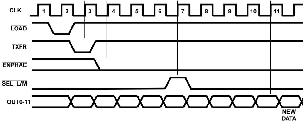
FIGURE 3. I/O TIMING
