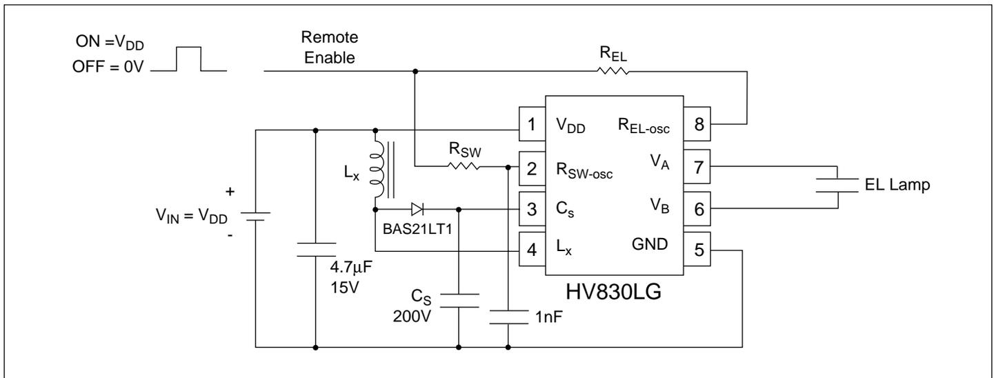
**Split Supply Configuration Using a Single Cell (1.5V) Battery**
