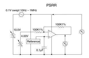
NOTE: Set Feedback Voltage so that  $V_{COMP} = V_{DIVIDE} \pm 1mV$  before connecting transformer
