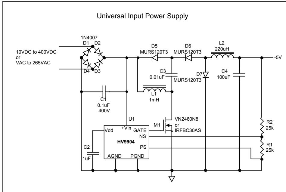
This circuit provides a non-isolated constant voltage output. The value of C4 capacitor controls the peak-to-peak ripple, which
