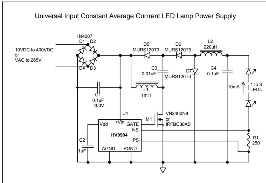
This circuit provides a constant average current output, which may be used to power LED lamps. The circuit maintains a constant average current and the value of C4 capacitor controls the peak-to-peak ripple, which decreases with increasing capacitor value. If
