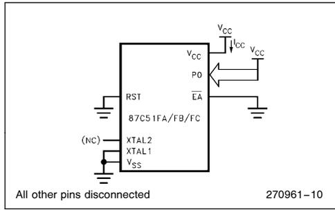
**Figure 9.  $I_{CC}$  Test Condition, Power Down Mode.
