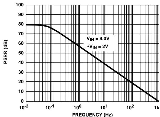
FIGURE 4. INPUT POWER SUPPLY REJECTION RATIO
