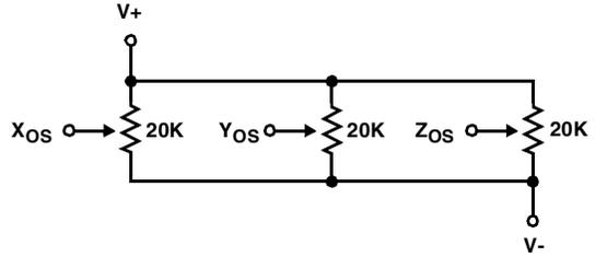
FIGURE 12. POTENTIOMETERS FOR TRIMMING OFFSET AND FEEDTHROUGH
