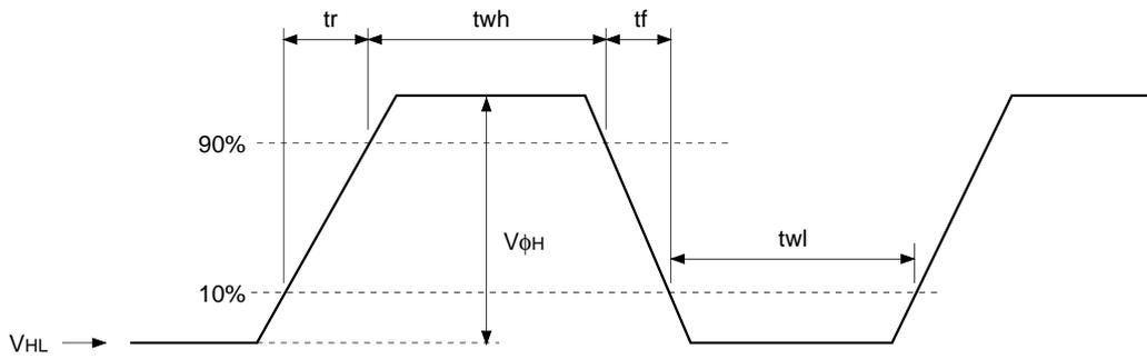
**(4) Reset gate clock waveform**
