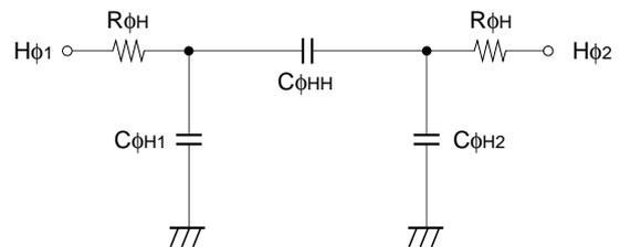
**Horizontal transfer clock equivalent circuit**
