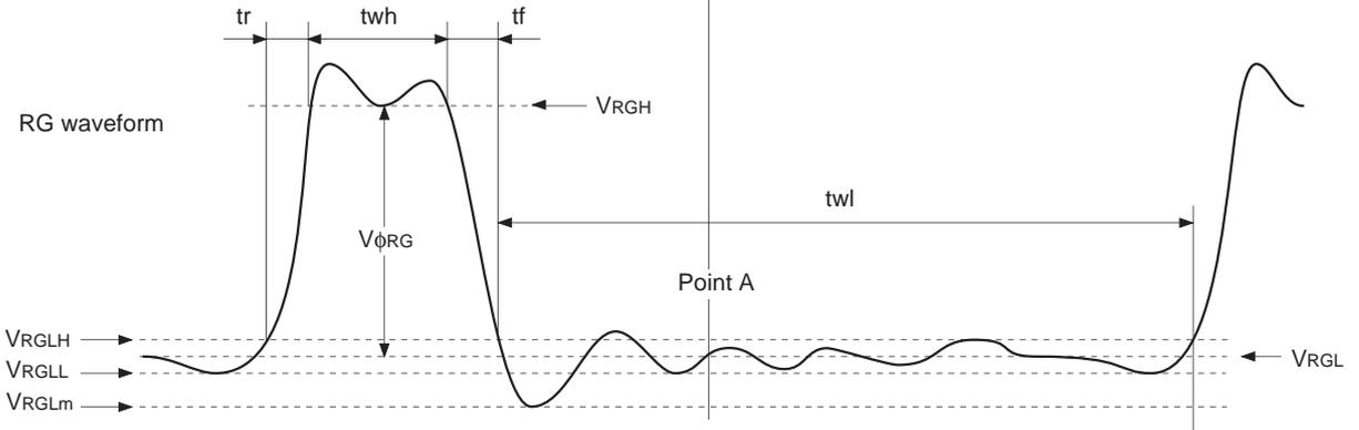
V<sub>RGLH</sub> is the maximum value and V<sub>RGLL</sub> is the minimum value of the coupling waveform during the period from Point A in the above diagram until the rising edge of RG.
