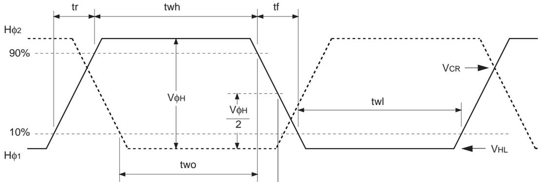
Cross-point voltage for the H $\phi_1$  rising side of the horizontal transfer clocks H $\phi_1$  and H $\phi_2$  waveforms is V<sub>CR</sub>. The overlap period for twh and twl of horizontal transfer clocks H $\phi_1$  and H $\phi_2$  is two.
