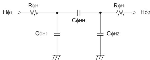
**Horizontal transfer clock equivalent circuit**
