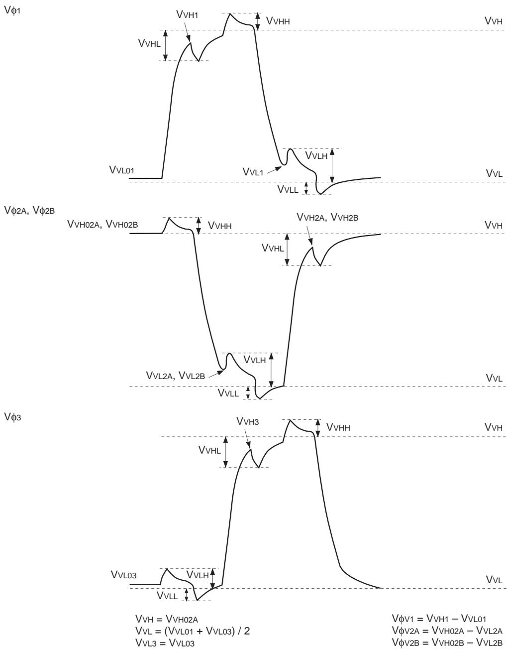
**(3) Horizontal transfer clock waveform**
